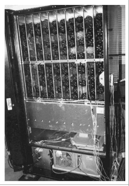
Coolers are one of the hardest pieces of equipment to repair, but yet one of the easiest to retrofit with a GRS 2100. This picture is of a typical single door cooler before the Cube is slid inside.
